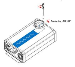
(2) Secure the screws of the LCD unit to the inverter.
