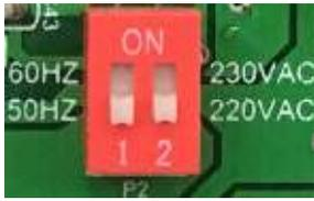
When the dial switch 1 is placed to the ON side, the output frequency is 60Hz, otherwise it is 50Hz,
