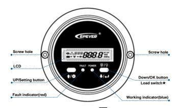
★In the real-time interface, long press for 2 seconds to turn off the load(default on); long-press it again for 2 seconds to turn on the load.
