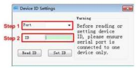
Caution: Only one of the controllers' IDs can be set at each time. Follow the same procedure to set the rest of the controllers.
