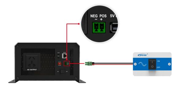
Connect the 3.81-2P green socket on the remote switch cable to the 3.81-2P green base on the product's side. Turn off the local toggle switch, and the remote switch will control the inverter's on/off.
