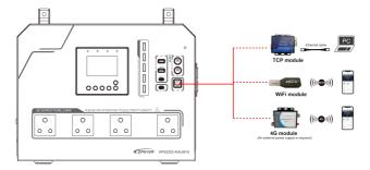
Note: The HPS-AHL is designed with a built-in Bluetooth module. After turning on the phone Bluetooth switch, the end-users can remotely monitor the HPS-AHL or set the parameters through the APP. For detailed settings, refer to the Solar Guardian APP user manual.
