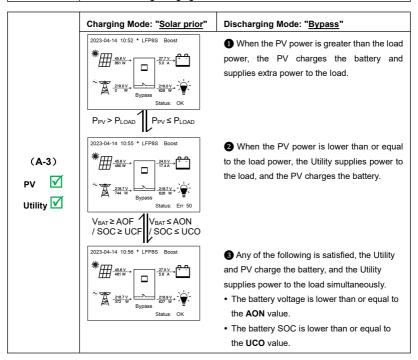
Note: When the battery voltage is greater than or equal to the AOF value, or the battery SOC is greater than or equal to the UCF value, the working mode returns to state 2. Working mode 2/3 are distinguished only by the difference in utility power. For working mode 2, the utility will not charge the battery, and for working mode 3, the utility charges the battery.
