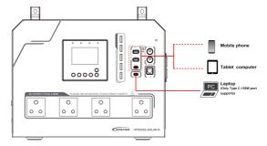
Charging the mobile phone, tablet computer, or laptop by the 5VDC/3A or USB-C (100W PD) port.
