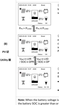
Regardless of the input and output sources, the working mode is as follows.
