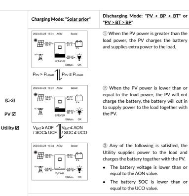
Note: When the battery voltage is greater than or equal to the AOF value, or the battery SOC is greater than or equal to the UCF value, the working mode returns to state @.
