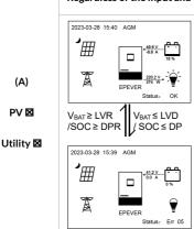
Regardless of the input and output sources, the working mode is as follows.
