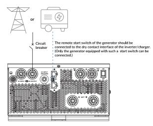
**Dry contact interface:** The dry contact interface can turn on/off the generator and is connected parallel with the generator's switch.
