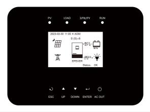
The display screen can be viewed clearly when the angle between the end-user's Tip horizontal sight and the display screen is within 90°. If the angle exceeds 90°, the information on the display screen cannot be viewed clearly.
