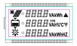
**Note:** The LCD can be viewed clearly when the angle between the end-user's horizontal sight and the LCD is within 90°. If the angle exceeds 90°, the information on the LCD cannot be viewed clearly.
