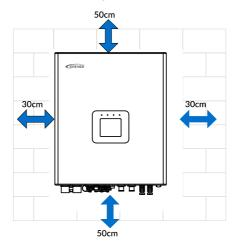
Step 2: Fix the wall hanger (included accessory) to the wall, and put the inverter/charger on it.
