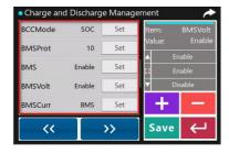
5. Click >>> to switch to the "Charge and Discharge Management" interface and set BCCMode, BMSProt, BMS, BMSVolt and BMSCurr. After the settings are complete, click Save to issue new parameters.
