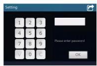
2. Enter the correct password (by default 000000) on the input interface, and click or to enter the "Setting Options" interface.
