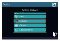
Slide up and down on the current interface, and click System to enter the system parameter setting interface.
