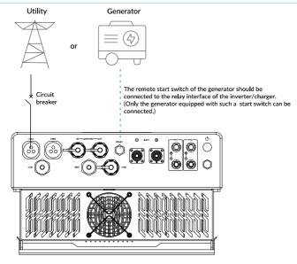
**Dry contact interface:** The dry contact interface can turn on/off the generator and is connected parallel with the generator's switch.
