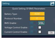
3. Select the "Battery Type" and "Protocol Number" and "SOC or VOL" according the actual situation, and click OK to return to the password input page. When selecting "Battery Type" as "AGM, GEL or FLD," "SOC or VOL" is displayed as VOL by default, and the "Protocol Number" is hidden. Only when the "Battery Type" is selected as lithium battery will the "Protocol Number" appear.
