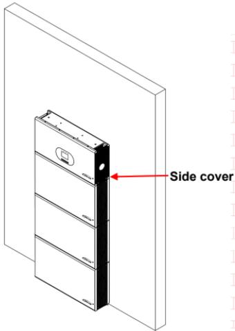
8 (Optional) When more than 3 battery packs are connected, it is recommended to install them into 2 columns (to avoid high stacking, which is inconvenient for maintenance in the future ), the two columns of battery packs are connected through the battery positive and negative power cables, and the RS485 communication cable, please refer to [6.2 Internal Wiring of the Energy Storage System](#).
