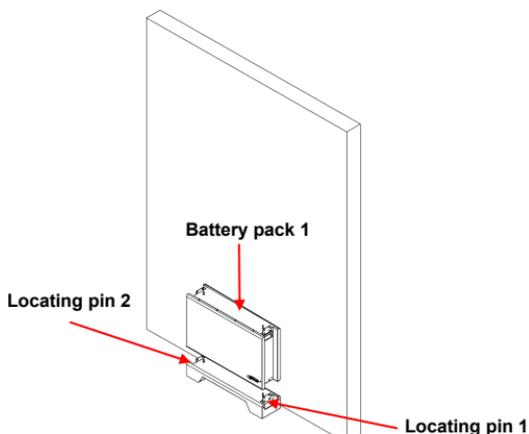
③ Stack the rest battery packs and the inverter in sequence on the fixed base, tighten the connecting pieces on the side with screws.
