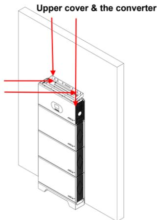
5 (Optional) When more than 3 battery packs are connected, 2 columns need to be installed (a single fixed base can only withstand up to 3 battery packs), the two columns of battery packs are connected through the battery positive and negative power cables, and the RS485 communication cable, please refer to [6.2 Internal Wiring of the Energy Storage System](#).
