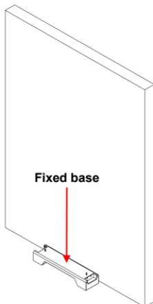
② Align the first battery pack with the locating pins and place it on the fixed base.
