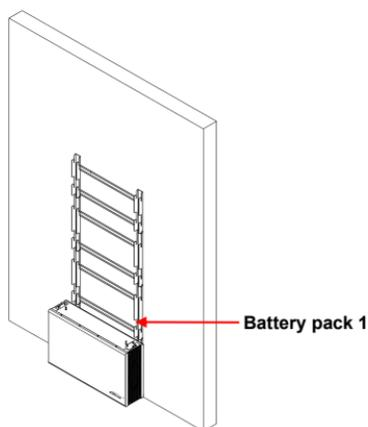
6 Stack the rest battery packs and the inverter in sequence on the wall mounting bracket, tighten the connecting pieces on the side with screws.
