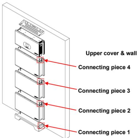
④ Fix the upper cover and wall with 2PCS M8\*50 expansion bolts, and fix the upper cover and the inverter with 2PCS M8\*16 hexagonal screws.
