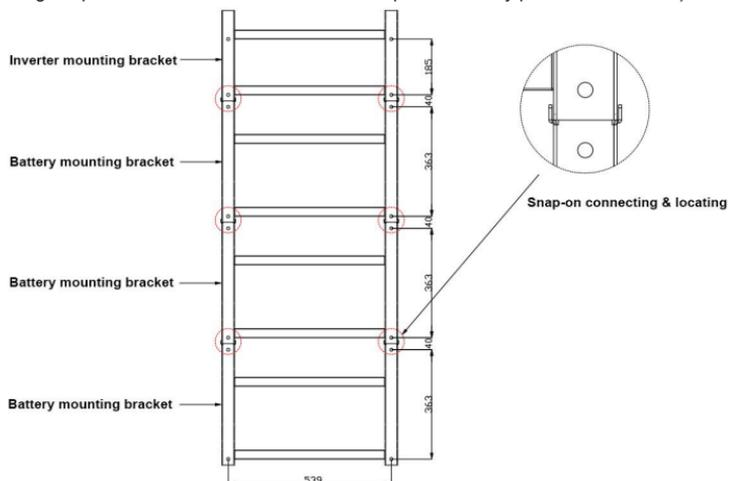
3 Use 4PCS M8\*50 expansion bolts to fix the battery mounting bracket to a wall that meets the installation requirements.
