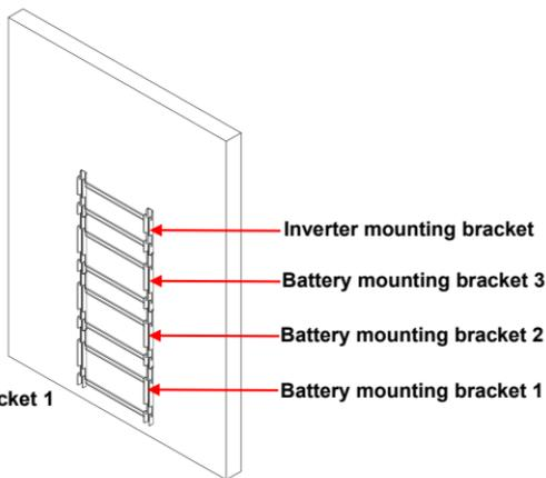
5 Install the first battery pack on battery mounting bracket 1.
