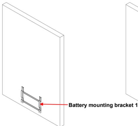
4 Install the rest battery packs and the inverter in sequence on the wall.
