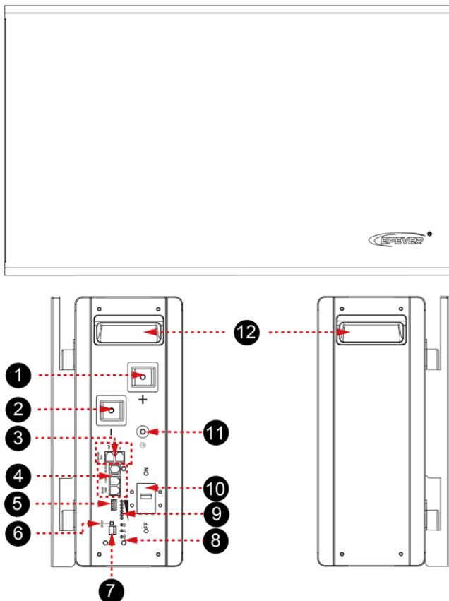
**Note:** The lithium battery pack appearance is illustrated above with the LFP5KWH51.2V-HP20 as an example.
