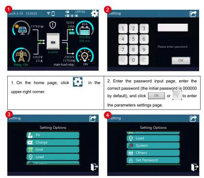
The parameters settings page includes: PV (PV parameters settings), Charge (battery charge control parameters settings), Grid (Grid parameters settings), Load (Load parameters settings), System (System parameters settings), Others (Other parameters settings) and password setting.
