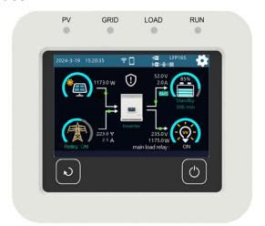
Note: The display screen can be viewed clearly when the angle between the end-user's horizontal sight and the display screen is within 90°. If the angle exceeds 90°, the information on the display screen cannot be viewed clearly.
