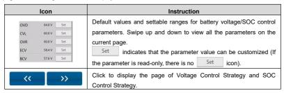
Note: For the content and operation methods of the parameters settings area on the right, please refer to the introduction of "1. PV (PV parameters settings)."
