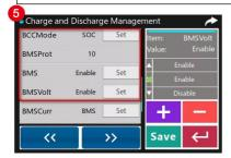
5. Click >>> to switch to the "Charge and Discharge Management" page and set "BCCMode (Battery Charging Control Mode), BMSProt (BMS Protocol), BMS (BMS Enable), and BMSVolt (BMS Voltage Control)." After the settings are complete, click Save to issue new parameter value.
