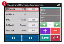
5. Click >>> to switch to the "Charge and Discharge Management" page and set "BCCMode (Battery Charging Control Mode)." After the settings are complete, click Save to issue new parameters.
