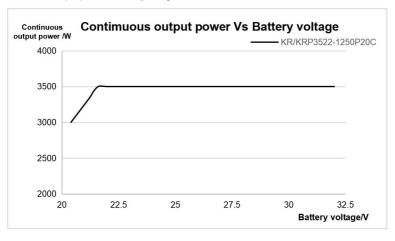
The parameters are measured in the condition of 48V/25 °C.
