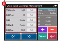
5. Click >>> to switch to the "Charge and Discharge Management" page and set "BCCMode (Battery Charging Control Mode), BMSProt (BMS Protocol), BMS (BMS Enable), BMSVolt (BMS Voltage Control), BMSCurr (BMS Current Control)." After the settings are complete, click Save to issue new parameters.
