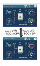
When the PV power is lower than or equal to the load power, the PV will not charge the battery, the battery will cut in to supply power to the load together with the PV.
