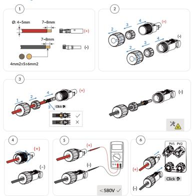
**Step 1:** Select the appropriate cable type and specification according to Section <u>3.4 Port cable description</u>. And remove the cable connectors from the PV cables. It is recommended to differentiate the positive and negative terminals with different colors.
