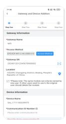
Step 3: On the "Gateway and Device Addition" interface, fill in the "Device Name" (or use default name of the APP) and "Communication ID Number<sup>(2)</sup>", click "Select Products Series" to enter the device selection interface.
