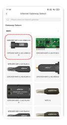
Step 2: Select "EPEVER WiFi 2.4G USB3.0 D", it will automatically return to the "Gateway and Device Addition" interface in <u>Step 5</u>. Scan the QR code<sup>(1)</sup> on the gateway label or manually enter the 22-digit gateway SN; Select the "Location" (optional), check the information prompt.
