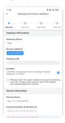
Step 1: Enter "Gateway and Device Addition" interface, fill in the "Gateway Name" (or use default name of the APP), click "Access Method" to enter "Internet Gateway Select" interface.
