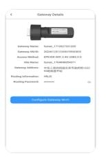
**Step 3:** Enter the "Gateway Details" interface to view the related gateway information. After the network configuration of the WiFi module is completed, the WiFi name and password of the router are displayed. Click the icon to switch to displaying the password in plain text to verify the correctness. Click "Configure Gateway WiFi" to enter the network configuration process, the network configuration of the WiFi module is completed or corrected.
